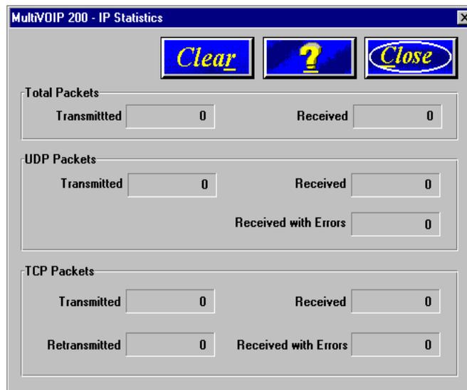
UDP makes use of the port concept and has no measures for flow control, reliability, or error recovery. It is used when the full services of TCP are not required, and the reliability measures must be assumed by another layer.
