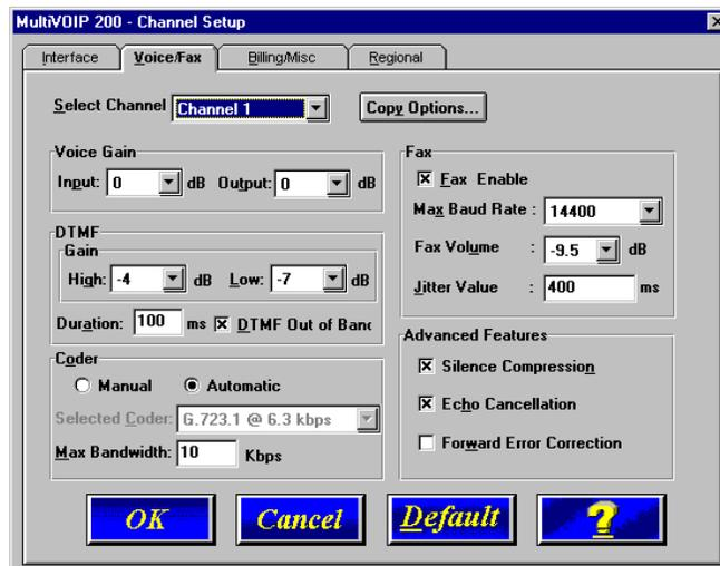
In our typical application, you would configure the corporate office channel parameters for an FXO interface. With this interface, the defaults for the Dialing Options and the type of Disconnect could remain as the defaults. For the remote branch office, the interface would be FXS with Loop Start being used in most cases.
