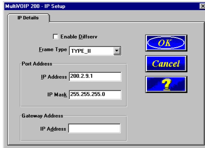
With **IP Setup** dialog box displayed you can change the status of differential services, the Ethernet Frame Type, the IP address and IP Mask of your H.323 endpoint, and the Gateway Address of the IP address of the device connected to the Internet.
