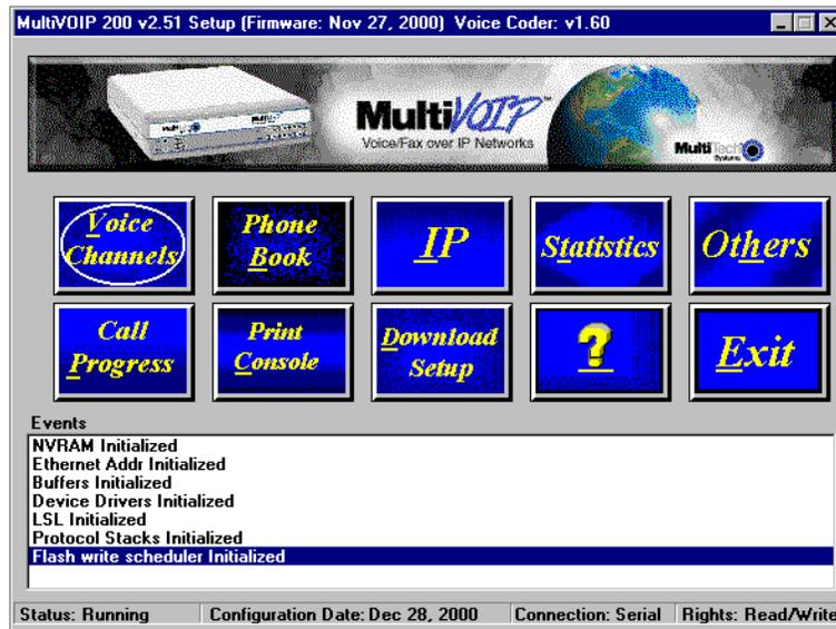
10. After you have changed the configuration of the remote MultiVOIP 200, click **Download Setup** to update the configuration. The remote MultiVOIP 200 will be brought down, the new configuration written to the unit, and the unit will reboot.
