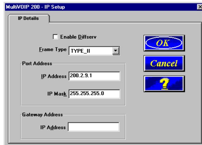
Click (check) the **Enable Diffserv** box if you have routers that support Diffserv (sometimes called IP Precedence). This feature gives priority to voice packets so they are not delayed because of large data files being downloaded.
