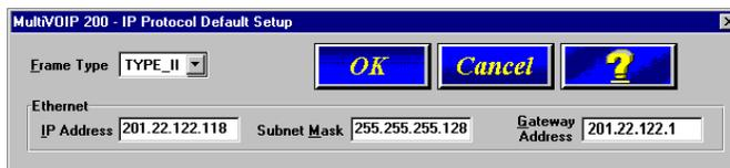
For your corporate MultiVOIP, the Ethernet Frame Type is Type II, the IP Address is 201.22.122.118, the Subnet Mask Address is 255.255.255.128, and the router Gateway Address is 201.22.122.1. The remote branch office would have the same Frame Type, a LAN IP address of 206.25.124.120 and a
